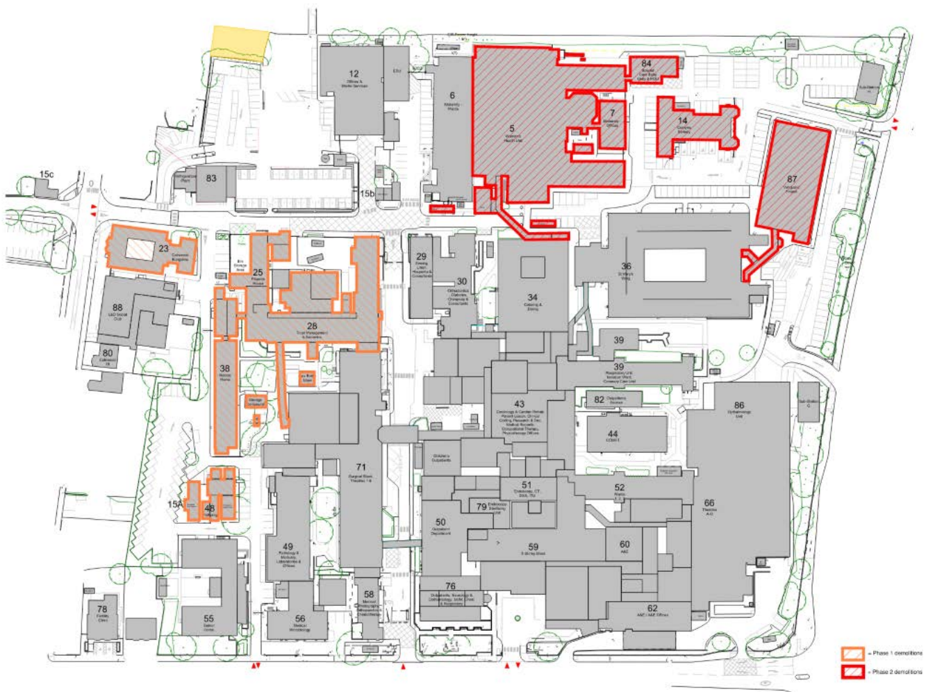
Figure 4.7: Phase 1 and 2 site demolition plan
